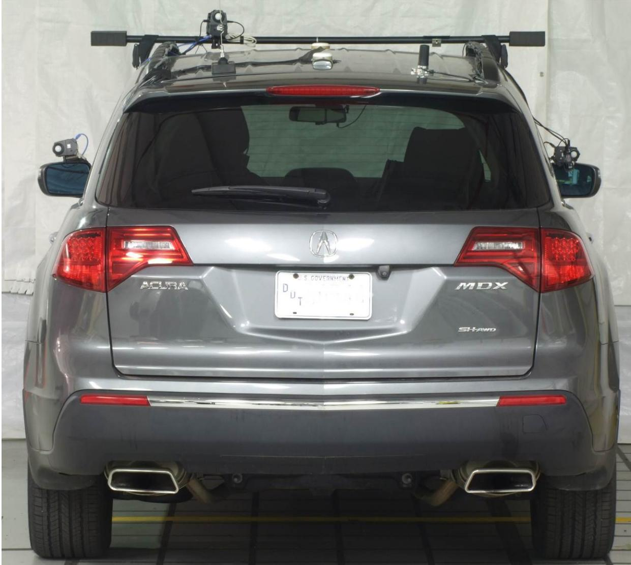
**Figure 28.** SUV DAS (Acura MDX) Rear
