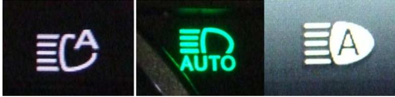
**Figure 1.** Headlighting System Automatic Mode Telltales Used to Indicate ADB Activation
