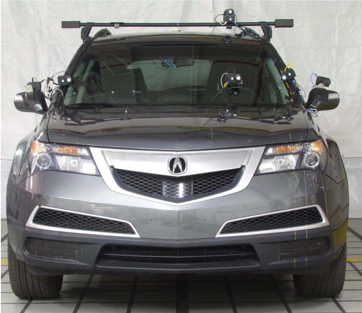
**Figure 27.** SUV DAS (Acura MDX) Front
