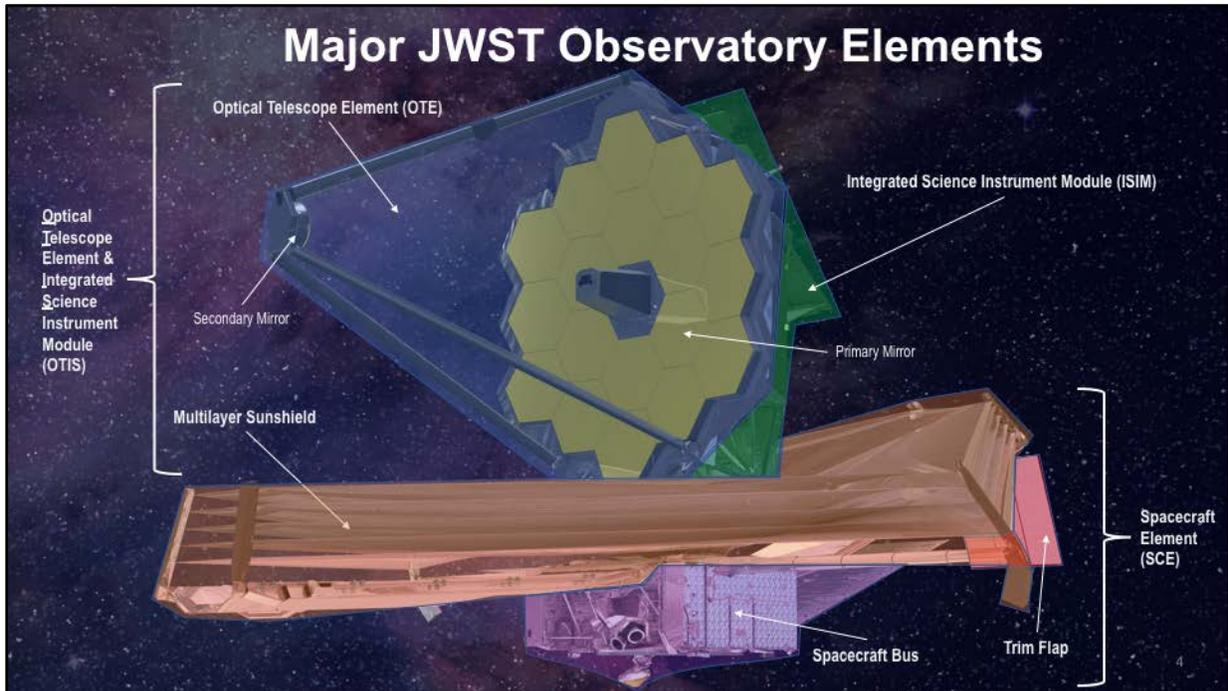
There are two primary elements of the JWST observatory. The first is the combined Optical Telescope Element and Integrated Science Module, or OTIS. The second is the Spacecraft Element (SCE), which is the combined Spacecraft Bus, Trim Flap, and Multilayer Sunshield.
